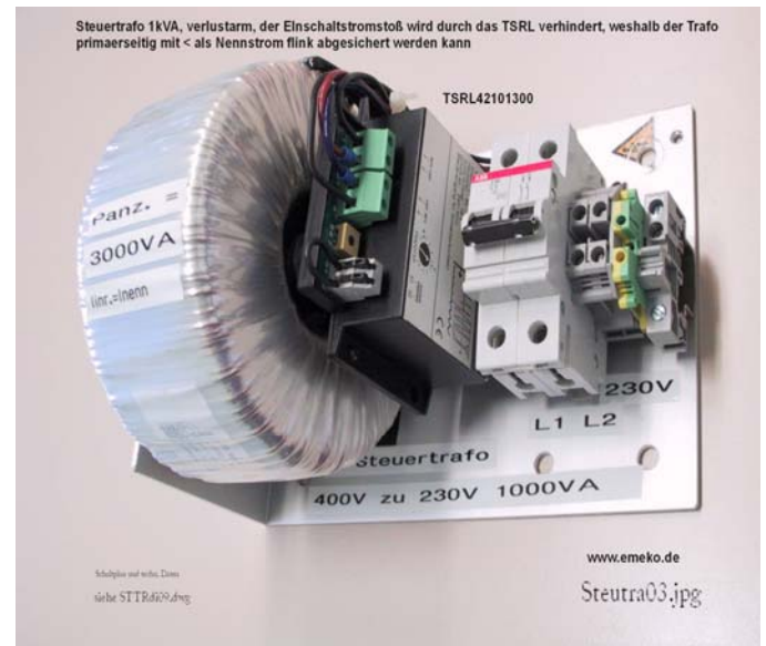
Picture 4. Transformer switch on without inrush current peaks
