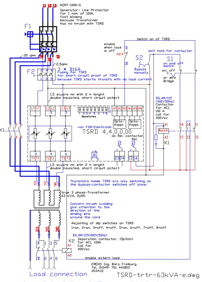
when capacitive loads like big power line filters are connected at the output, or when other single phase transformer are connected at the output, a separation contacter K2 is needed.
