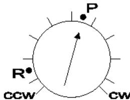
**Toroidal core transformers:** Use the setting nearly R. ( nine o'clock)
