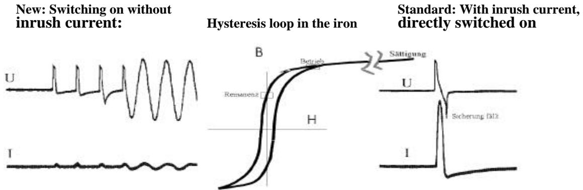
With Transformer Switch Relay, premagnetised and switched on opposite to the direction of premagnetized remnance polarity without inrush current at the nominal or open circuit current.
